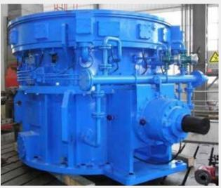
多点传动式立磨减速机 Reducer of heavy vertical grinding mill
