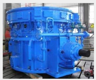
传统式立磨减速机 Reducer of heavy vertical grinding mill
