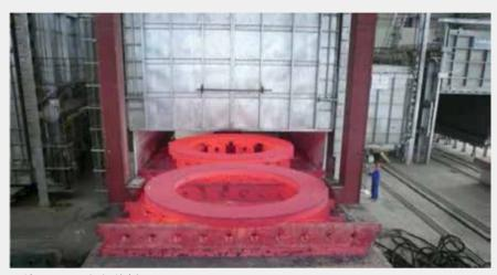
三峡 700MW 机组镜板 Three Gorges 700MW water power station unit runner plate
