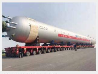
镇海石化 2400 吨沸腾床加氢反应器 2400t fluidized bed hydrogenation cracking reactor for Zhenhai Petrochemical
