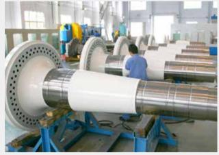
风力发电机主轴 Wind Power Generator Main Shaft
