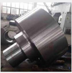
F 级燃气轮机后轴头 Rear shaft end of F-class gas turbine
