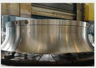
白鹤滩 1000MW 水轮机分瓣式不锈钢下环 Split stainless steel band of Baihetan 1000MW water turbine
