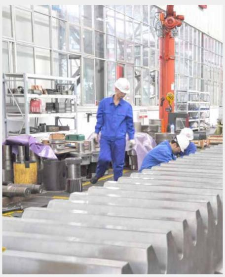
二重装备研制的世界最大的三峡升船机齿条 EHEC Developed the World Largest Ship Elevator Gear Rack for Three Gorge Project Gorge Project
