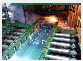
广西银海铝 3300+2850 铝板带热连轧机 Guangxi Yinhai 3300+2850 aluminum plate hot strip rolling mill
