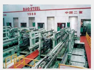
宝钢 1550mm 冷轧主轧线 1550mm Cold rolling mill for Bao Steel
