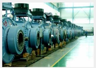
1.5MW 风力发电增速机 Speed-increasing gearbox for 1.5MW wind mill
