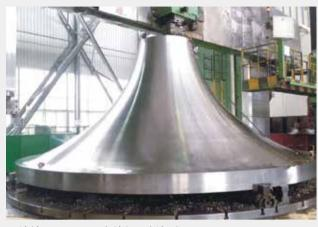
三峡地下 700MW 水轮机不锈钢上冠 Three Gorge Underground Power Station 700MW Water Turbine Crown of Stainless Steel
