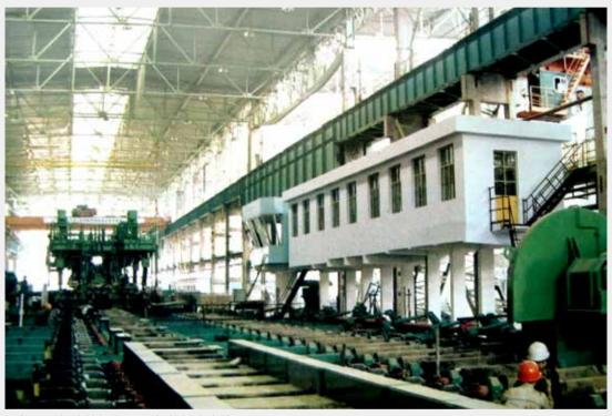
马钢异型坯连铸机和 H 型钢轧机生产线 Blank/beam continuous casting machine and H-section beam steel rolling mill for Maanshan Iron & Steel Co.
