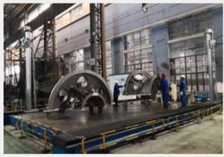
80MW/GE-6F 压气机及透平缸 80MW/GE-6F Compressor and turbine cylinders
