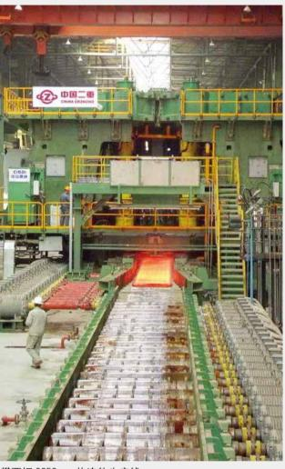
攀西钢 2050mm 热连轧生产线 2050mm hot strip rolling production line for Panxi Steel
