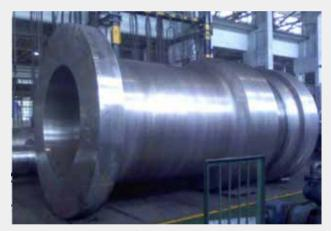
混流式 650MW 糯扎渡整锻主轴锻件 Monoblock Forging of the Main Shaft for Nuozhadu mixed-flow 650MW Hydropower Generating Unit
