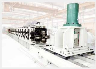
纵梁辊型部件 Roll Forming Unit for Beam
