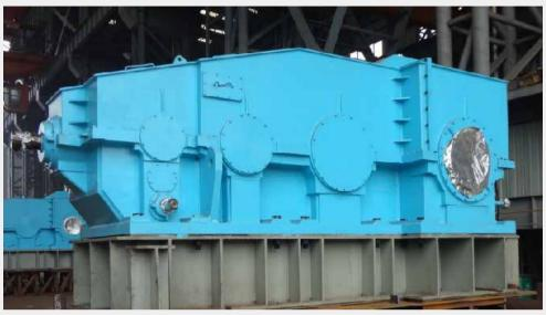
亭子口升船机齿轮箱 —SCJ 1650 Gear box (SCJ 1650) of ship elevator for Tingzikou project
