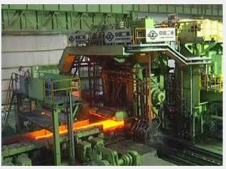
河北安丰 1780mm 热连轧生产线 1780mm hot strip rolling production line for Hebei Anfeng
