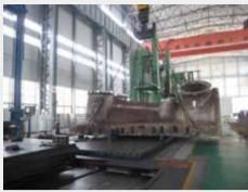
(高中压外缸上半 4-1) (Upper half of HIP outer casing 4-1)
