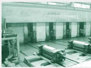
鞍钢 1680mm 酸轧联合机组 Hot strip rolling mill and pickling line for Anshan Steel
