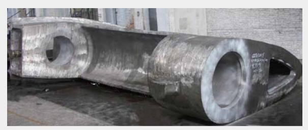
172000M3LNG 船挂舵臂 172000M3LNG Ship Rudder Arm
