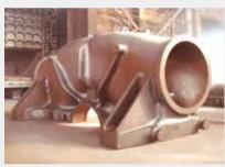
(中压排汽外缸上半 1-3) (Upper half of IP exhaust outer casing 1-3)
