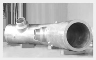
AP1000 主管道热锻 A AP1000 main pipeline hot section A
