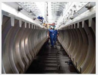
二重装备研制的向家坝升船机螺母柱 EHEC Developed the Ship Elevator Nut Post for Xiangjiaba Project
