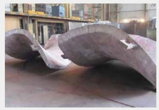
美国勒丁顿 312MW 抽水蓄能水轮机不锈钢叶片 American Ludington 312MW Pumped Storage Water Turbine Blade of Stainless Steel
