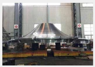
白鹤滩 1000MW 水轮机分瓣式不锈钢上冠 Split stainless steel crown of Baihetan 1000MW water turbine
