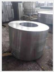
F 级燃气轮机拉杆螺母 Nuts of the tie rod of F-class gas turbine
