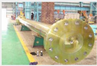
船轴类 Forgings for Marine Shafts Application
