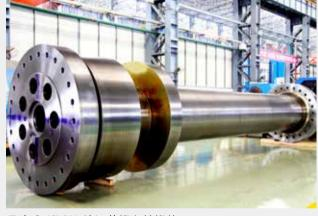
贯流式 40MW 峡江整锻主轴锻件 Monoblock Forging of the Main Shaft for Xiajiang Outer Gate Barrel Type 40MWHydropower Generating Unit
