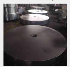
F 级燃气轮机轮盘 Disc of F-class gas turbine
