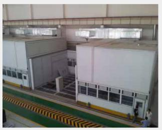
移动组合形成密闭喷漆室 Moving combination to form a closed spray chamber
