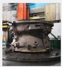
270MW-312MW 透平缸 270MW-312MW Turbo Cylinder
