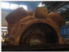
(中压排汽外缸下半 3-3) (Lower half of IP exhaust hood (outer casing) 3-3)
