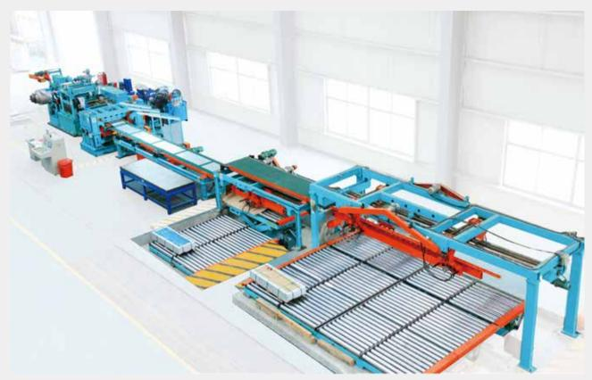
RS-2×800 飞剪生产线 Cut to Length Rotary Shear Production Line
