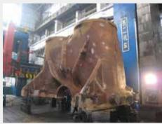
(中压排汽外缸上半 4-3) (Upper half of IP exhaust hood (outer casing) 4-3)
