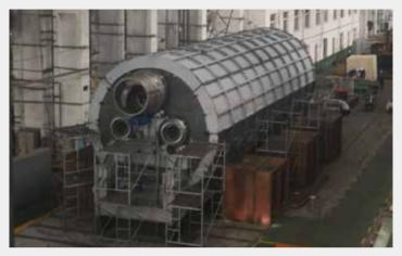
100 吨 / 日垃圾熔融裂解处理设备 100 tons/day waste fusion cracking processing equipment
