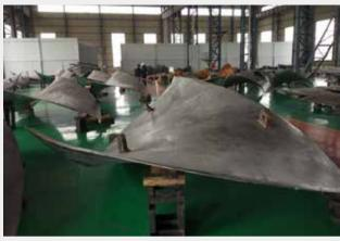
白鹤滩 1000MW 水轮机不锈钢叶片 Bai He Tan Power Station 1000MW Water Turbine Blade of Stainless Steel
