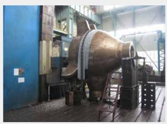
(CPR1000 铸造泵壳 5) CPR1000MW Cast pump casing 5)
