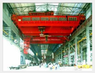
550t 锻造四梁桥式起重机 550t 4-beam forging overhead crane
