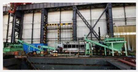
2 万吨 / 年撬装式油基钻屑热解吸处理设备 20,000 t/a Skid-mounted Oil-based Drillings Thermal Desorption Treatment Equipment
