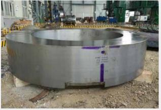
乌东德 850MW 水电机组下法兰锻件 Lower flange forging of Wudongde 850 MW hydro-power generator set
