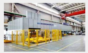
RS $-3 \times 1850$  汽车外板飞剪生产线 Cut to Length Rotary Shear Production Line for Automobile Outer Panel
