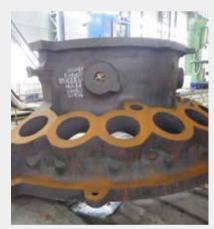
270MW-312MW 燃烧室 270MW-312MW Combustion Chamber
