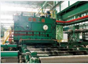
获得国家专利的滚切式定尺剪 The sizing shear-the national patent obtained.
