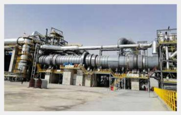
年产 60 万吨粉煤热解回转反应炉 Annual output of 600,000 tons of pulverized coal pyrolysis slewing reactor
