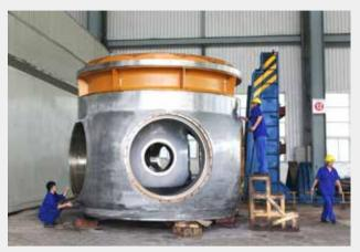
葛洲坝 175MW 水轮机转轮体 Gezhou Dam 175MW Water Turbine Runner
