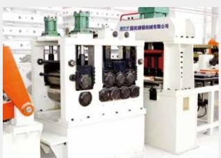
纵梁校平剪切部件 Leveling and Cutting Unit for Beam
