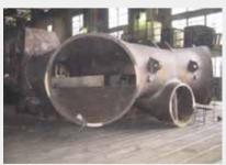
(中压排汽外缸下半 1-4) (Lower half of IP exhaust outer casing 1-4)
