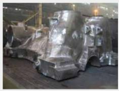
(高中压外缸下半 3-2) (Lower half of HIP outer casing 3-2)
