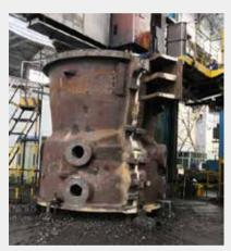
270MW-312MW 燃烧室兼压气机缸 270MW-312MW Combustion Chamber & concurrently functioning as an air compressor cylinder
