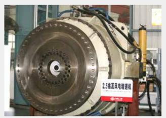
2.5MW 风电增速机 Speed-increasing gearbox for 2.5MW wind mill
