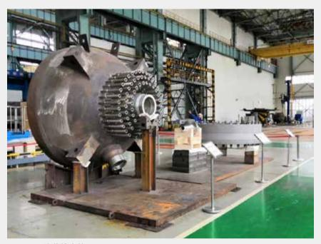
CAP1400 堆芯补水箱 CAP1400 Core Makeup Tank
