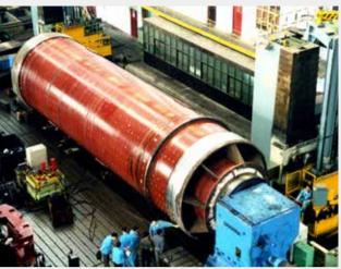
大型水泥磨筒体 The heavy duty shell for the cement grinding mill
