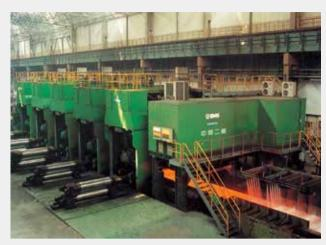
邯钢 1680mm 连铸连轧机 1680mm CC-CR mill for Handan I&S Co
