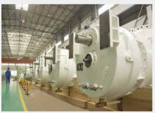
1.0MW 风力发电增速机 Speed-increasing gearbox for 1.0MW wind mill
