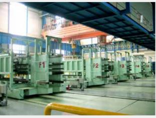
天铁 1720mm 冷轧机组 1720mm cold rolling mill for Tianjin Tiantie Metallurgy Group Co.LTD
