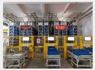
小件自动化立体仓库 Small work pieces automated stereoscopic warehouse
