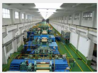
1450mm 连续酸洗平整机组 1450mm continous pickling temper mill
