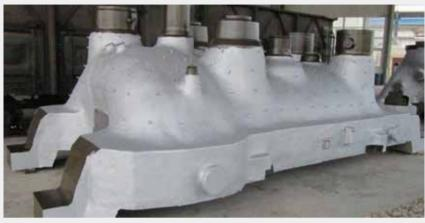
300MW 汽轮机缸体 — 高中压外缸 300MW Steam Turbine Cylinder Body -High & Intermediate Pressure Outer Cylinder
