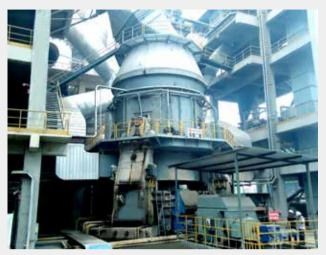
日产 6000 吨大型原料立磨 Large raw material vertical mill of 6000 tons per
