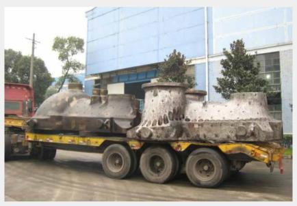
330MW 汽轮机缸体 — 中压外缸 330MW Steam Turbine Cylinder Body - Intermediate Pressure Outer Cylinder
