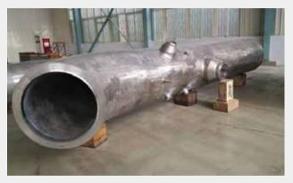
华龙一号主管道热段 A Main pipeline hot section A for Hualong No. 1 Project
