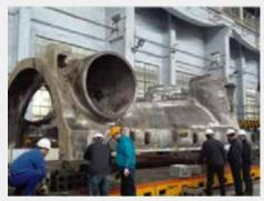
(高中压外缸下半 4-2) (Lower half of HIP outer casing 4-2)
