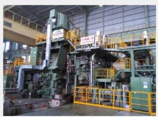
宝钢湛江 2250mm 热连轧生产线 Zhanjiang 2250mm hot strip rolling production line for Baoshan Iron & Steel Co.
