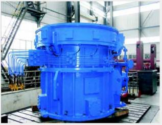
大型立磨减速机 Reducer of heavy vertical grinding mill
