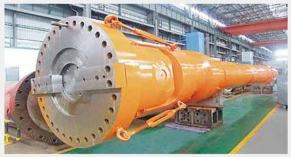
湘钢 5000mm 热轧主传动万向接轴 Xiang Steel 5000mm Hot Mill Main Drive Universal Spindle
