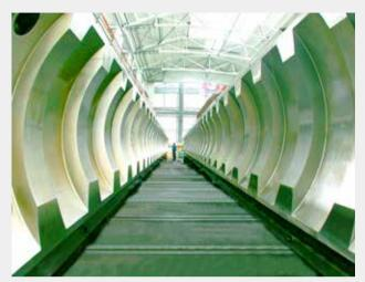
二重装备研制的世界最大的三峡升船机螺母柱 EHEC Developed the World Largest Ship Elevator Nut Post for Three Gorge Project
