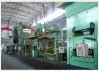
一汽 EXY125MN 热模锻曲轴前梁自动生产线 EXY 125MN Front axle and crankshaft die forging press line
