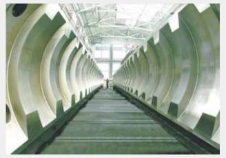
二重装备研制的世界最大的三峡升船机螺母柱 EHEC Developed the World Largest Ship Elevator Nut Post for Three Gorge Project
