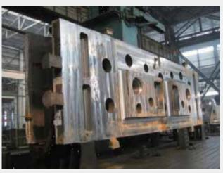
活动横梁侧梁体 Side beam body of the moving crosshead
