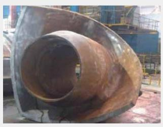
32 万吨油轮后轴壳 Oil carrier of 320,000 tons Rear Axle Housing
