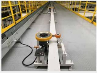
摩擦输送设备 Friction conveyors
