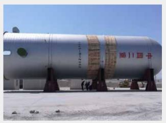
恒力石化 600 万吨 / 年柴油加氢裂化装置加氢反应器 Diesel hydrogenation cracking reactor with a capacity of 6 million tons/year for Hengli Petrochemical
