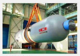
上海石化渣油加氢反应器 Shanghai Petrochemical Residue Hydrogenation Reactor
