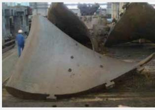
三峡地下 700MW 水轮机不锈钢叶片 Three Gorge Underground Power Station 700MW Water Turbine Blade of Stainless Steel
