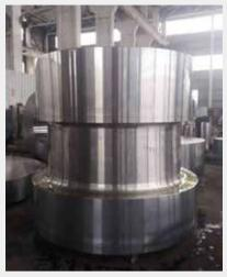
F 级燃气轮机前轴头 Front shaft end of F-class gas turbine
