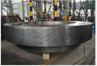
乌东德 850MW 水电机组推力头锻件 Thrust head forging of Wudongde 850 MW hydro-power generator set
