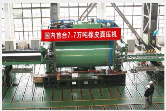
770MN 橡皮囊液压成形机 770MN rubber bladder hydraulic forming machine
