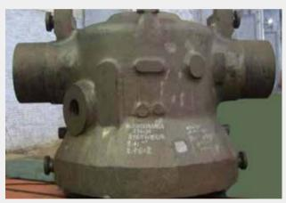
12%Cr 不锈钢高压进气端 12%Cr stainless steel HP air inlet end
