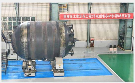
CAP1400 堆芯补水箱 CAP1400 Core Makeup Tank
