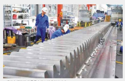
二重装备研制的世界最大的三峡升船机齿条 EHEC Developed the World Largest Ship Elevator Gear Rack for Three Gorge Project Gorge Project
