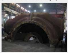
(中压排汽外缸上半 3-4) (Upper half of IP exhaust hood (outer casing) 3-4)
