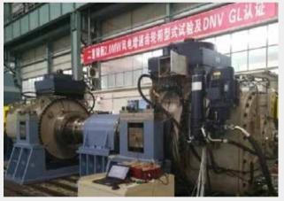
2.0MW 风电增速机 Speed-increasing gearbox for 2.0MW wind mill
