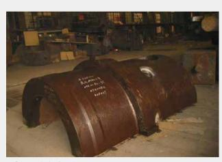
12%Cr 不锈钢高压缸 12%Cr stainless steel HP casing
