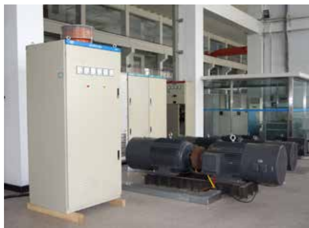
低压变频式试验机组 Test motor group for low-voltage adjustable frequency converter
