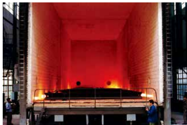
上海锅炉厂 30m × 7.5m × 8.5m 大型全纤维热处理炉 30m×7.5m×8.5m Large Size Whole Fiber Heat Processing Furnace of Shanghai Boiler Factory
