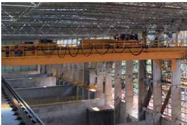
华新水泥崇德联合储库—全自动抓斗起重机（4台同轨） Huaxin Cement Chongde Joint Repository —Fully automatic crane (parallel arrangement of 4 garbage handling crane)
