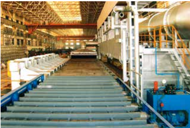
哈尔滨锅炉厂超超临界锅炉管屏整体高温固溶热处理生产线 Overall High Temperature Solid Solution Heat Treatment Production Line of The Supercritical Boiler Panel of Harbin Boiler Company Ltd.
