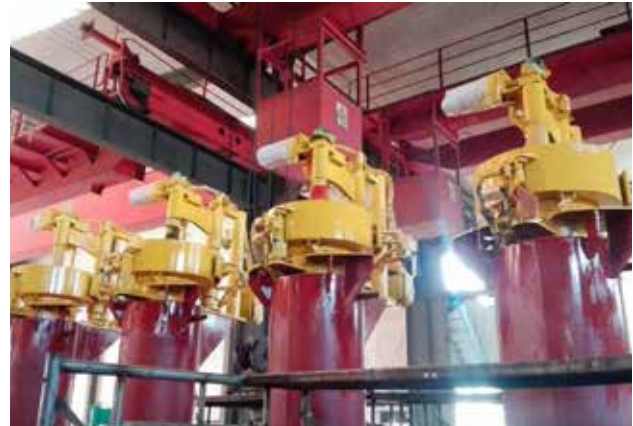
(20MPa~50MPa 级) 系列快开装置 CO 2 高压萃取釜 A Series of (20MPa~50MPa) quick opening devices for high pressure CO 2 extraction kettle
