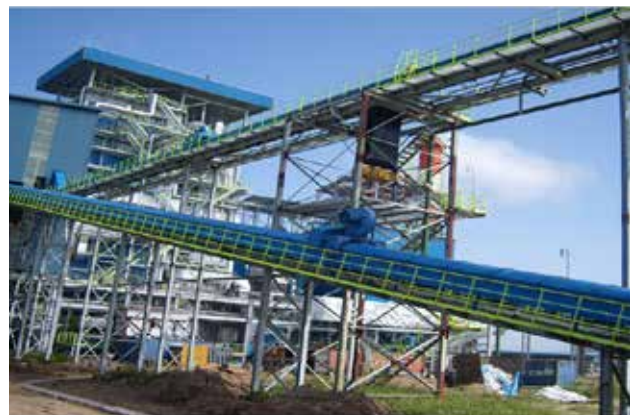
圭亚那糖厂 B1400 B2200 气垫式蔗渣输送机 B1400 B2200 Bagasse cushion type conveyor for Guyana Sugar Factory
