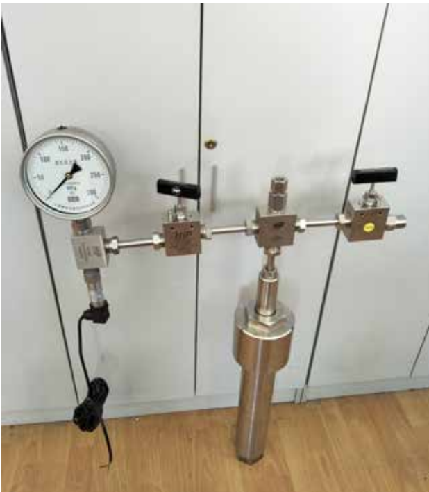
高温超高压反应釜，酸性氨热法生长高质量、大尺寸氮化镓单晶衬底的核心设备 High Temperature and Ultra High Pressure Reactor, Core Equipment for High Quality and Large Size GaN Single Crystal Substrates Produced by Acidic Ammonia Thermal Process
