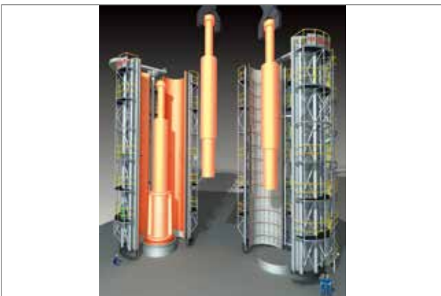
立式旋转开合式电阻热处理炉和立式旋转开合喷淋淬火装置 Vertical Revolve Retractable Resistance Heat Furnace & Vertical Revolve Retractable Spray Quenching Device
