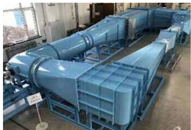
广州高澜节能有限公司试验系统大型闭式循环风洞 - 水换热系统 Large closed loop wind tunnel-water heat exchange system of Guangzhou Goaland Energy Conservation Tech Co., Ltd
