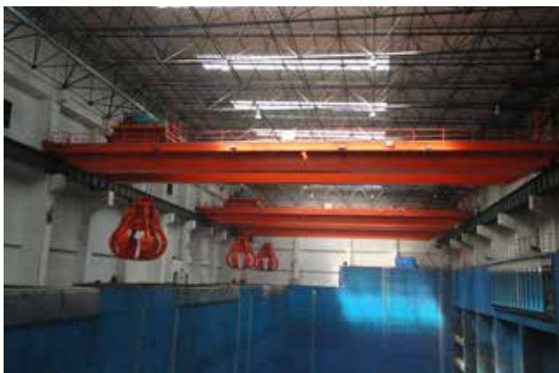
粤丰环保集团横沥项目—高级半自动控制垃圾抓斗起重机（3台同轨） Waste-to-Energy Project in Hengli Dongguan, China—High Level Semi-auto bridge crane (parallel arrangement of 3 garbage handling crane)
