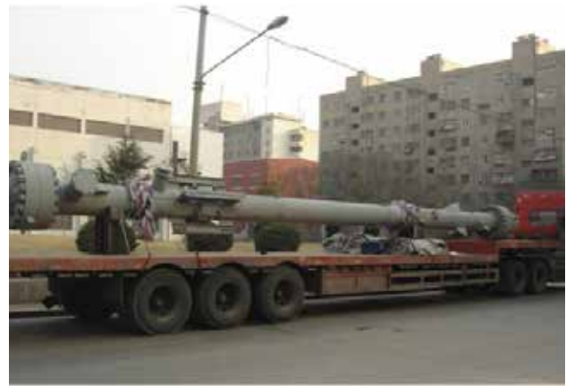
扬子巴斯夫公司固定管板式循环气冷却器 Fixed tube-sheet type circulating gas cooler of Yangzi petrochemical-basf co. LTD
