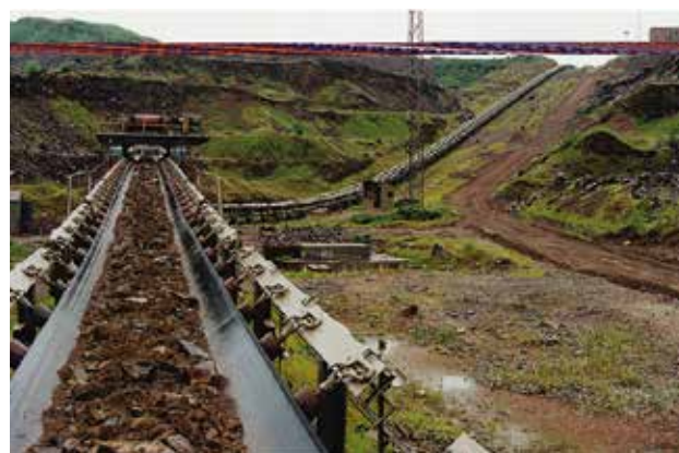
首钢水厂铁矿半连续排岩系统 Semi-continuous rock burden spreading system in Shuichang
