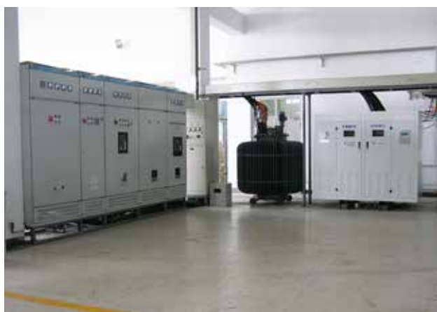
900kVA 无功及谐波发生源试验系统 900kVA reactive power and harmonic source system
